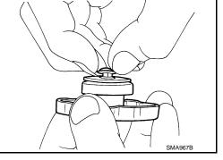
Check reservoir tank cap relief pressure.
