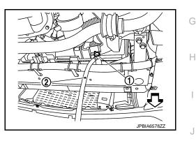
When draining all of engine coolant in the system, open water drain plugs on cylinder block. Refer to <u>EM-87, "Setting"</u>.
